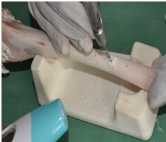
Figure 2: Temperature of conventional drill recorded with infrared thermometer
