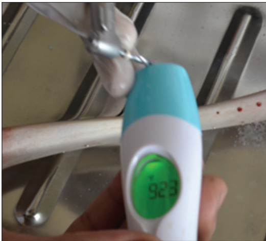
Figure 1: Temperature of trephine drill recorded with infrared thermometer
